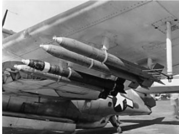
"Holy Moses" HVARs mounted on a TBF Avenger
